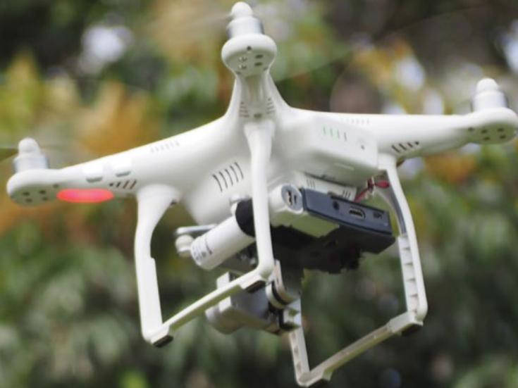
A drone fitted with a thermal camera. Photo: José Lahoz-Monfort
